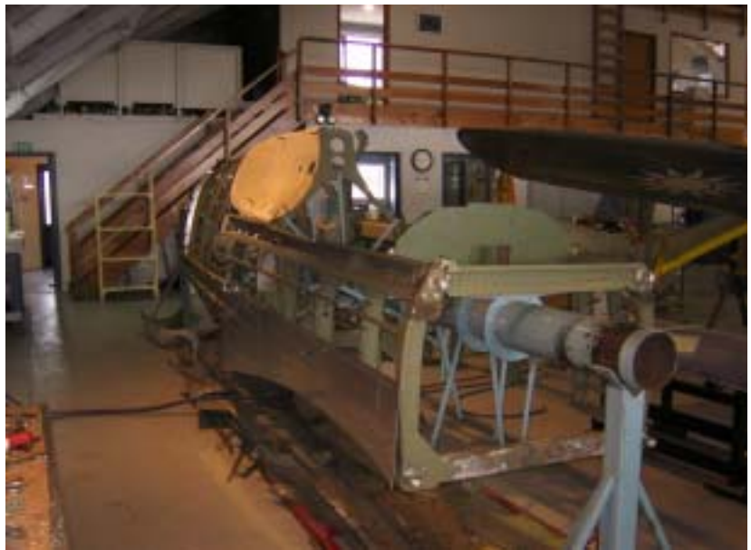
A29-414 fuse on the jig with first skins being pinned on.
