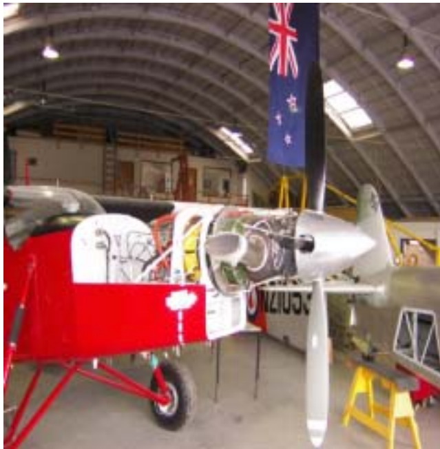
Porter engine and prop fitted.
