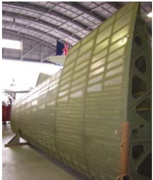
The second Lockheed 10 wing is out of the jig
