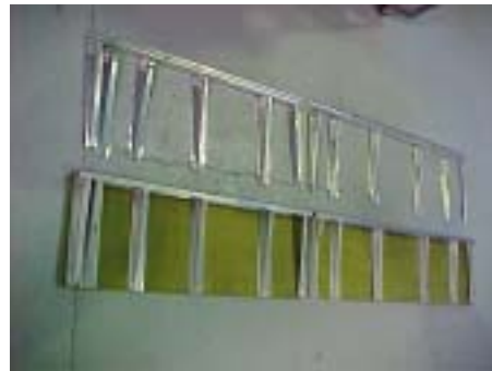
Ammo Bay door parts waiting to be assembled
