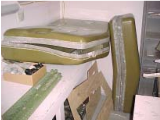
Fuel tanks ready for final assembly
