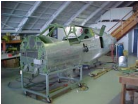
Jerry's fuselage with 2-seat conversion underway
