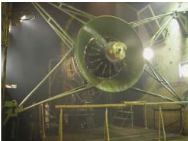
The engine running on the test stand
