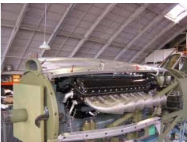
Cowl assembly underway - engine in.
